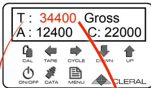
Deploy the auxiliary axle and adjust its pressure gauge to 30 psi. The weight transferred to axle B changes the total weight.
